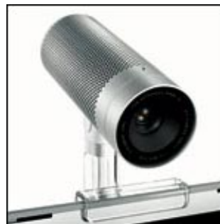
Figure 1: The Apple iSight webcam used in our vision system. For gesture recognition, the iSight is particularly well-suited since it sits on top of the user’s monitor, at eye level. By placing the camera directly in front of the user, motions can be directed at the computer screen rather than at some off-axis camera, allowing for a more intuitive interface.
