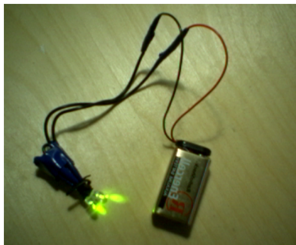
Figure 5: We constructed an LED finger thimble out of four green LED lights. The LEDs are solder together in a serial circuit and connected to a 9V battery pack.
