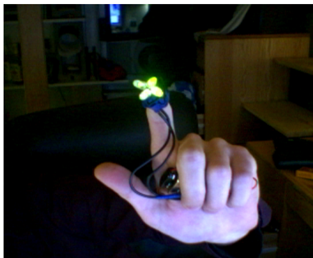
Figure 2: The four LED thimble attached to a user's index finger. The four LEDs are splayed to distribute the light intensity over a range of angles. This allows a bright light to be seen by the camera no matter what orientation the user prefers to keep their finger.
