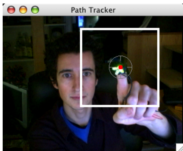
Figure 6: Here we see the search window used for our tracking optimization overlaid on the video display. If the light source is not found by searching this smaller area, the entire video frame is searched in the next iteration.
